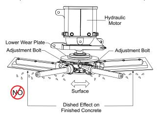
Figure 34. Incorrect Spider Plate Alignment
